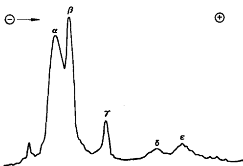
Fig. 1. Densitometric tracing of ATPase in 10 % acrylamide gel containing 0.1 % SDS. Electrophoresis was carried out for 3 h at 8 V/cm at room temperature.
